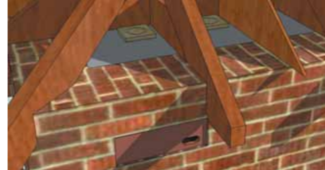
Illustration of an internal nest box, which can be built in to the structure of the building. © Dick Newell
